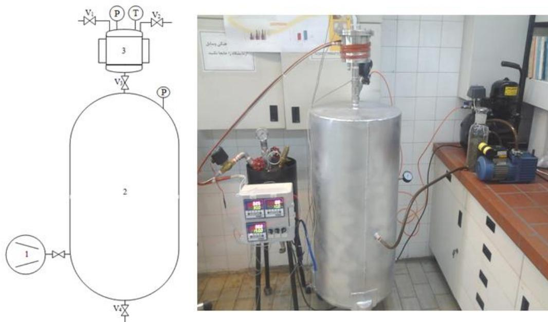
**Figure 2.** Instant Controlled Pressure Drop (DIC) apparatus. (1) Vacuum Pump; (2) Vacuum tank; (3) DIC treatment chamber; (V1) Steam inlet valve; (V2 and V4) Discharge valve, (V3) Pneumatic vacuum valve.
