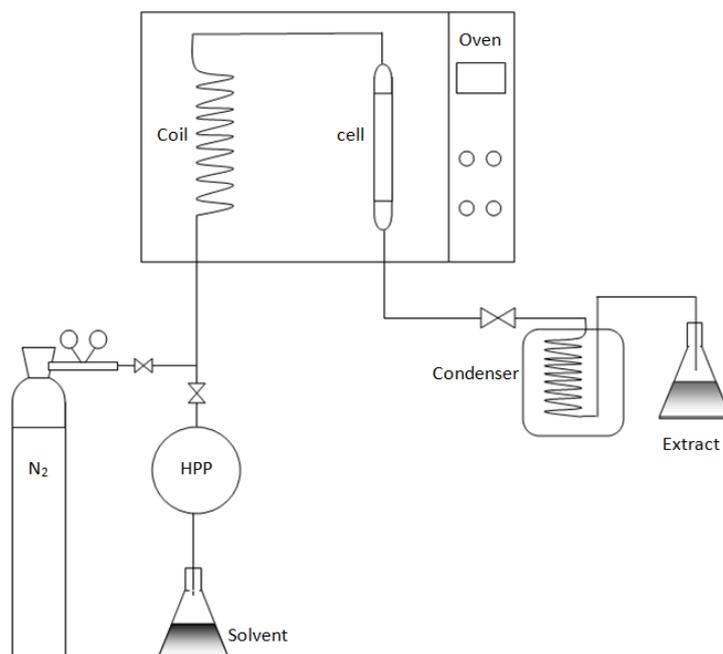
**Figure 1.** Schematic diagram of superheated solvent extraction apparatus. N<sub>2</sub>: Nitrogen capsule, HPP: High Pressure Pump.
