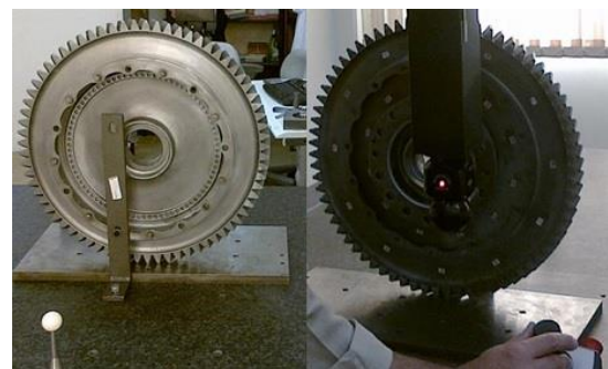
Fig. 4 disc dimension measurements by coordinate measurement machine (CMM)
