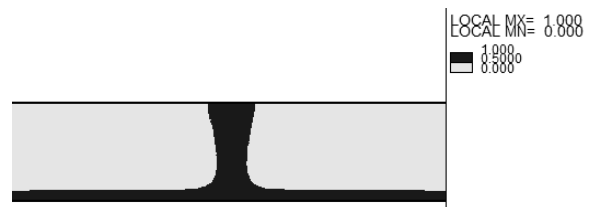
Fig. 5 STAR-CD 2D results for the case of water entrance from middle and top of the tank with 1m/s speed at 0.5s
