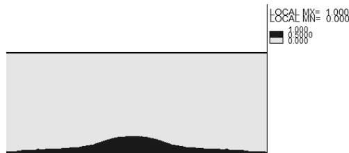
Fig. 2 STAR-CD 2D results for the case of water entrance from middle and bottom of the bed with 0.2m/s speed at 0.5s
