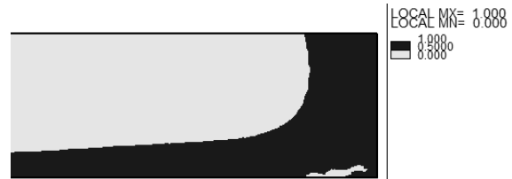
Fig. 7 STAR-CD 2D results for the case of water entrance from top edges of the tank with 1m/s speed at 0.5s (zoomed screen at right corner)
