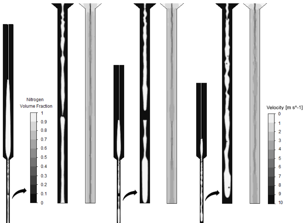
Fig. 5 Contours of Nitrogen volume fraction and velocity magnitude for three different mixing chamber lengths (12.7mm, 25.4mm and 50.8mm) inside the effervescent atomizer at GLR=0.08\% .
